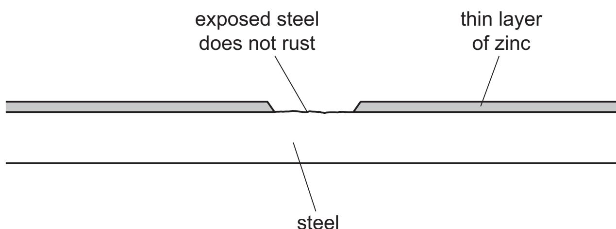
The piece of steel coated with zinc still did not rust but the copper-coated piece of steel rusted very rapidly.
